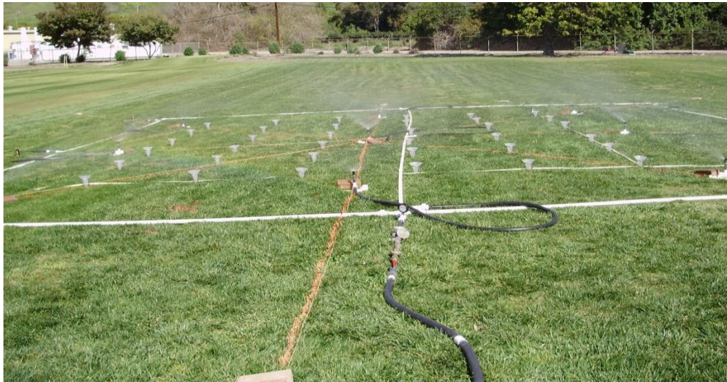
Figure 2. Test system with nozzles and catch cans. Point of connection for the system with pressure regulator, water meter and pressure gauge is in the forefront
