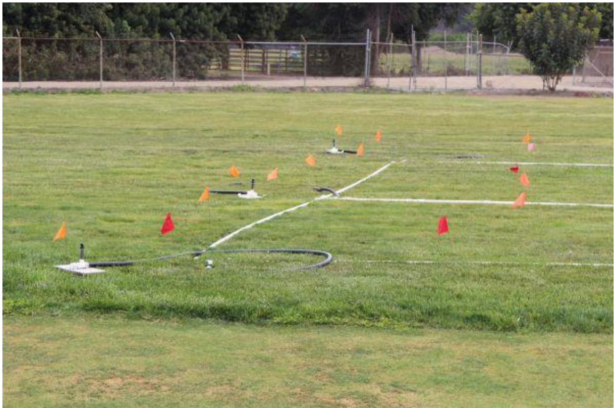
Figure 3. Sprinkler nozzles on shrub adapters mounted on movable platforms to setup the required nozzle spacings
